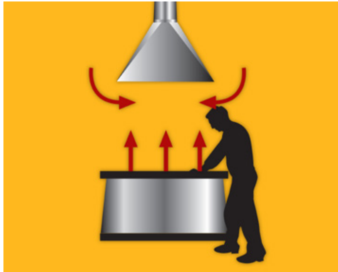
↑ Using an overhead hood may allow contaminated air to be pulled across the worker's breathing zone.
