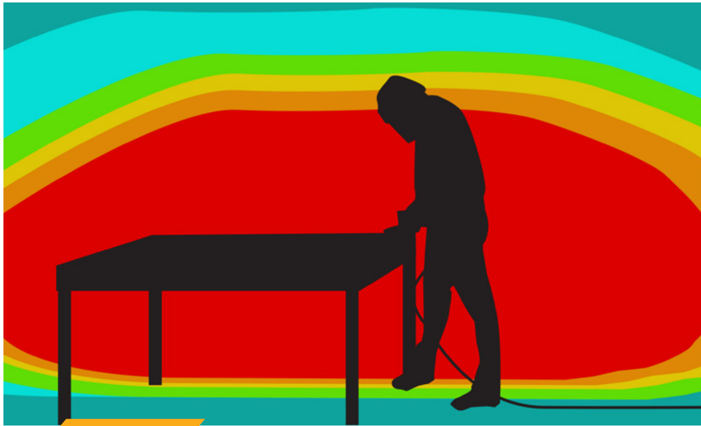
↑ A cross-flow collector's booth-wide velocity profile showing clean air pull across the worker's breathing zone. The red zone represents the highest air velocities.
